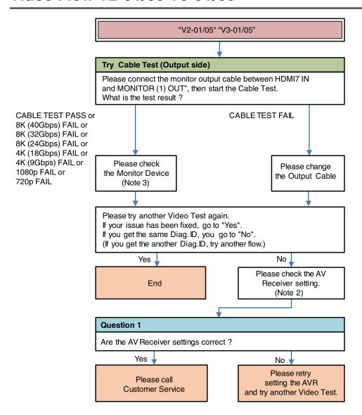
**Description "V\*-01"**: Miscommunication with Monitor at output terminal (HPD always low).
