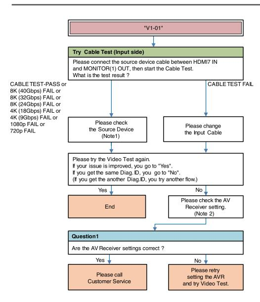
**Description "V1-01"**: Cannot detect the HDMI cable connected to the AVR input terminal (as detection of 5V from Source Device).
