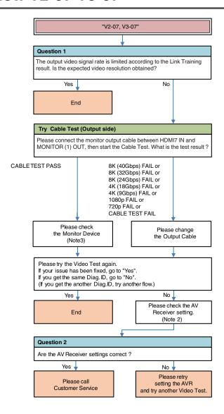
**Description "V2-07"**: FRL Link Training failed and Video signal format is limited to TMDS.
