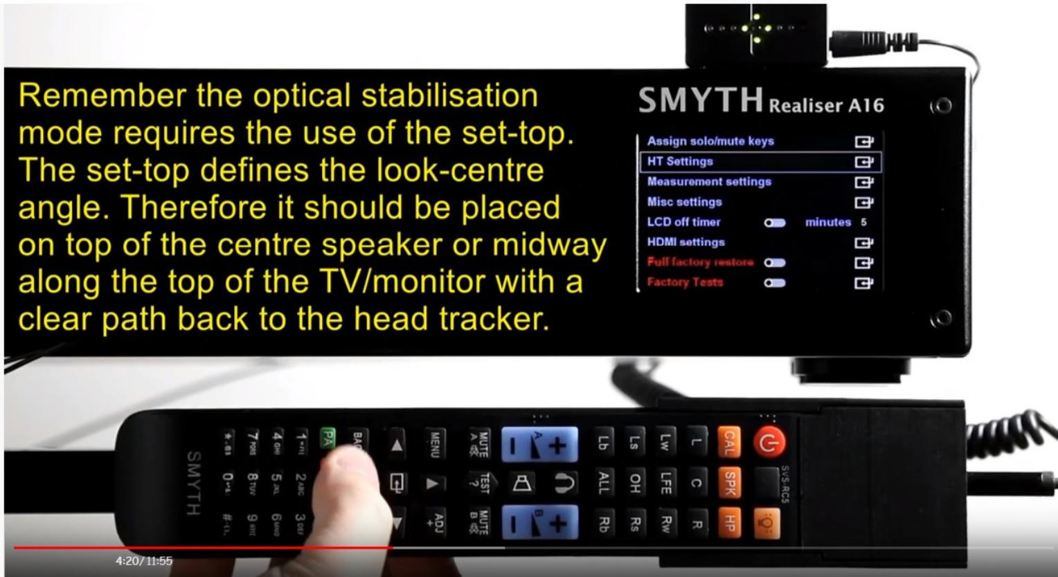
Remember the optical stabilisation mode requires the use of the set-top. The set-top defines the look-centre angle. Therefore it should be placed on top of the centre speaker or midway along the top of the TV/monitor with a clear path back to the head tracker.
