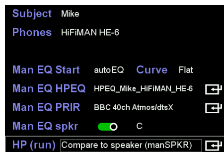
Figure 9-9 Configuration of HPEQ parameters for manual adjustment of an autoEQ filter, by comparing a virtual centre speaker from a measured PRIR against a real external loudspeaker as reference. The selected sub-band pink noise signals have a flat response curve.
