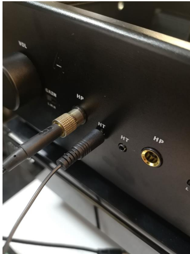
Figure 2-26: The Headphone and head-tracker head-top connected to the Realiser via the ports in the front panel.
