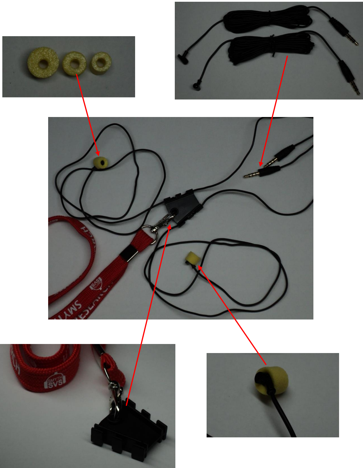
Figure 2-29: The binaural microphones used to create a PRIR.
