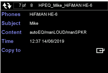
Figure 9-15 File information showing the contents of an HPEQ file in the recycle buffer. Three filters are available – autoEQ, manLOUD and manSPKR.
