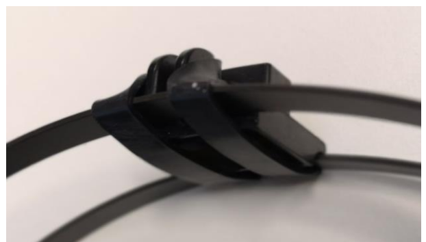
Figure 14-5: Mounting the head-top clip to the centre of the headphone band
