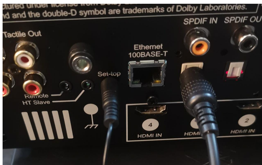
Figure 2-28: Set-Top connected to the Realiser via the Set-top port on the rear panel.
