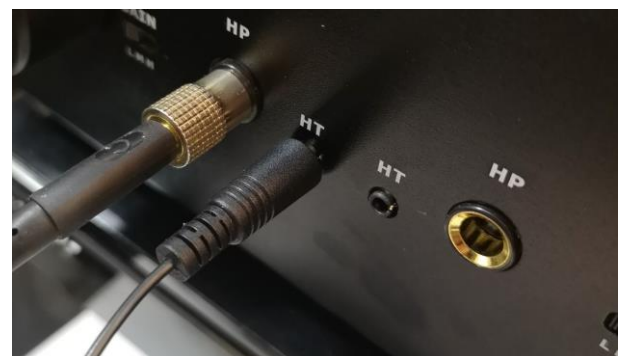
Figure 14-3: Connect the Head-top cable to appropriate HT port on the front panel of the A16
