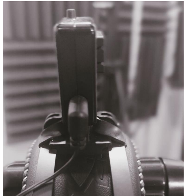
Figure 14-1: Connecting the 90-degree connector of the HT cable to the head-top device
