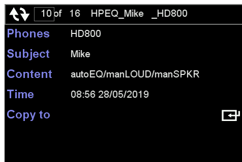
Figure 6-8 A HPEQ file in the recycle buffer showing three filters, autoEQ, manLOUD and manSPKR. Any of these filters can be chosen as the HPEQ filter within a preset.
