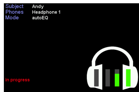
Figure 9-5: Automatic headphone EQ measurement showing the headphone signal and the recorded level in the right binaural microphone.
