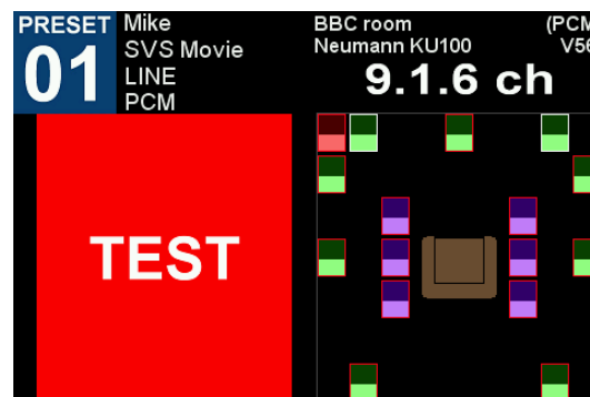
Figure 3-5 Mute mode: listening to groups of virtual speakers. Muted speakers are outlined in red, unmuted speakers in white. The Left and Right speakers are currently un-muted.
