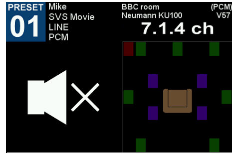
Figure 7-15: Muting the headphone output for User A using the MUTE key on the remote
