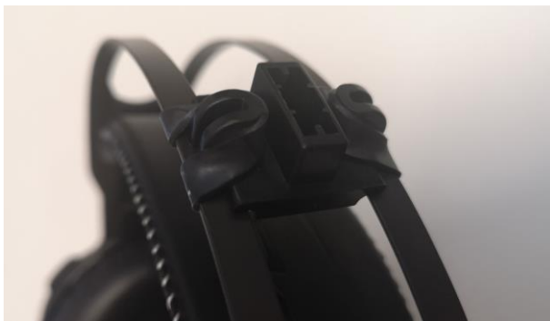
Figure 14-4: Mounting the head-top clip to headphones using a rubber band
