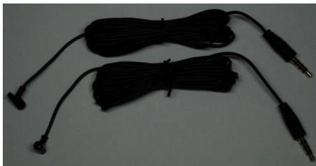
Figure 2-11: In-ear measurement microphones (one pair)
