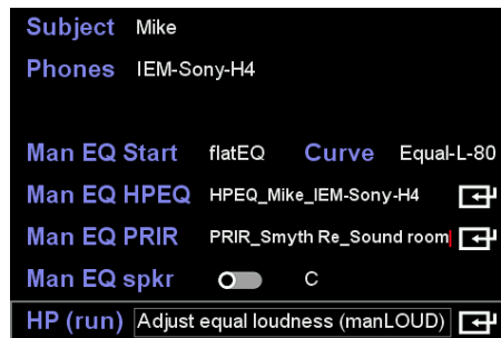
Figure 9-12 Configuration of the HPEQ menu options for manual EQ using the equal loudness technique. The flatEQ filter of the selected HPEQ file will be adjusted using an equal-loudness-80 curve for the sub-band noise signals, and the headphone signals will NOT be virtualised with a PRIR.
