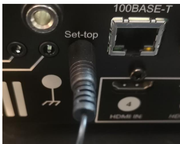
Figure 14-7: Connect the set-top cable to the Set-top port on the back panel of the A16
