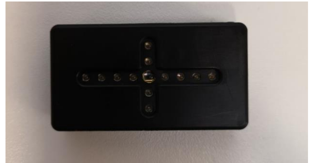
Figure 14-3: The Set-Top device that can be mounted in a central location such as a TV or video monitor
