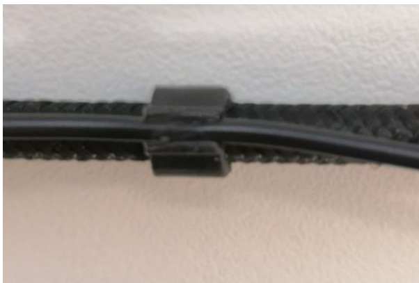
Figure 14-4: Connecting the head-top cable to the headphone cable using clips
