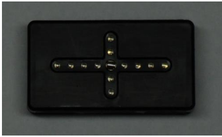
Figure 2-6: Set-top IR reference for head-tracking
