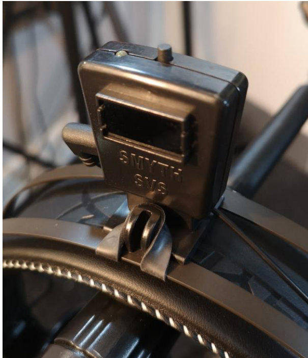
Figure 14-2: Mounting the head-top to the clip, front window facing forwards
