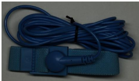
Figure 2-13: Grounding wrist-strap (used during microphone measurements to reduce body-induced hum)
