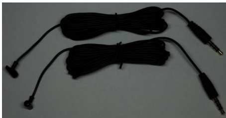
Figure 2-11: In-ear measurement microphones (one pair)
