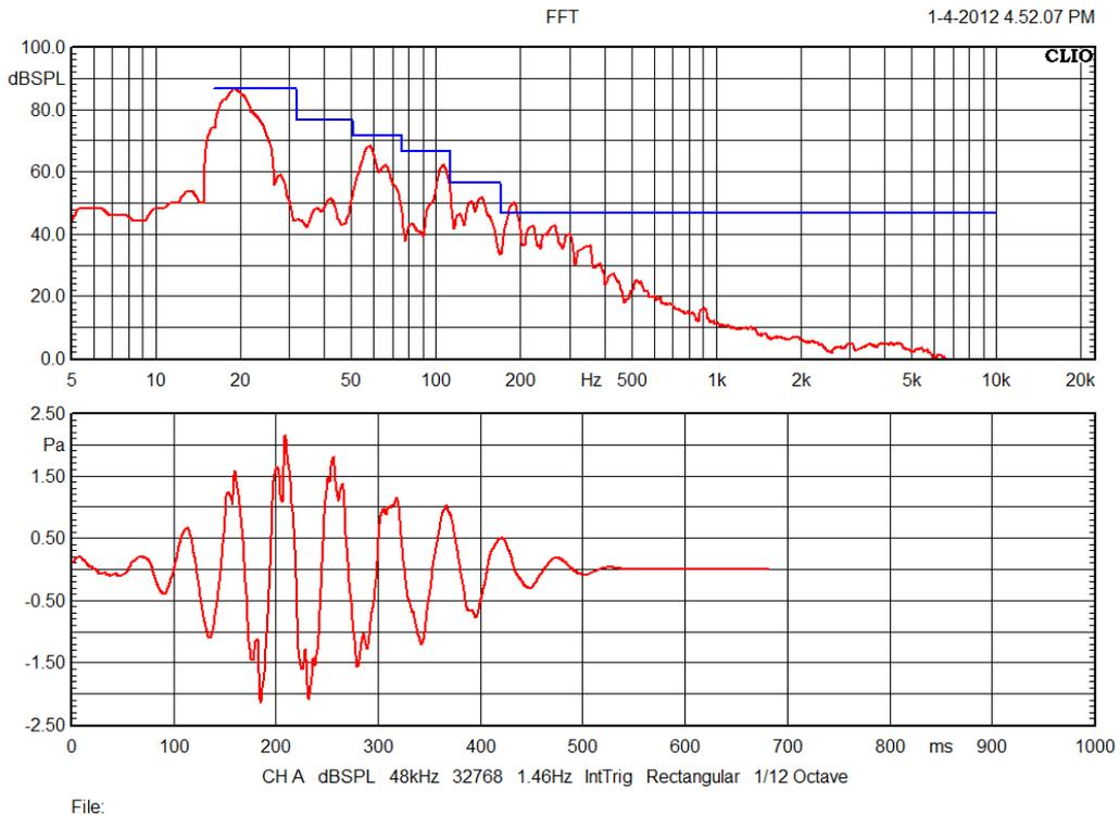
Figure 9: ACE-bass B2-50 - ANSI/CEA-2010 test @ 20 Hz
