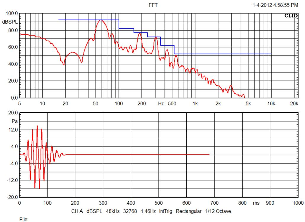
Figure 14: ACE-bass B2-50 - ANSI/CEA-2010 test @ 63 Hz
