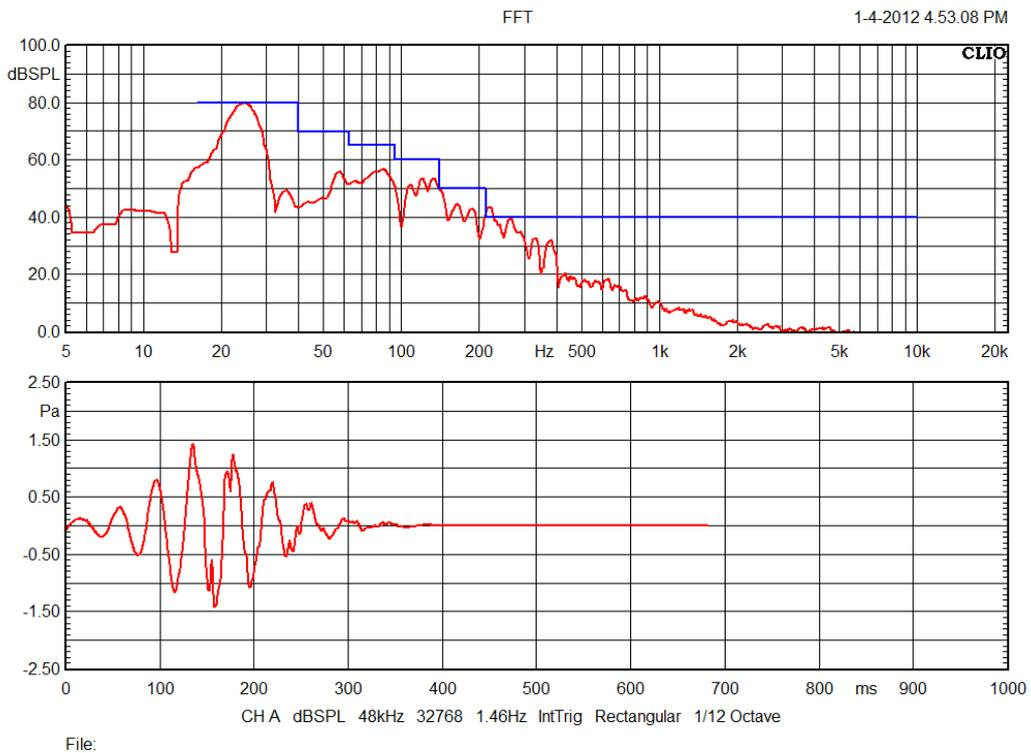
Figure 10: ACE-bass B2-50 - ANSI/CEA-2010 test @ 25 Hz
