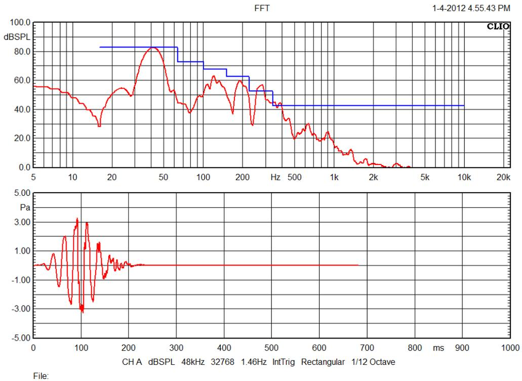
Figure 12: ACE-bass B2-50 - ANSI/CEA-2010 test @ 40 Hz
