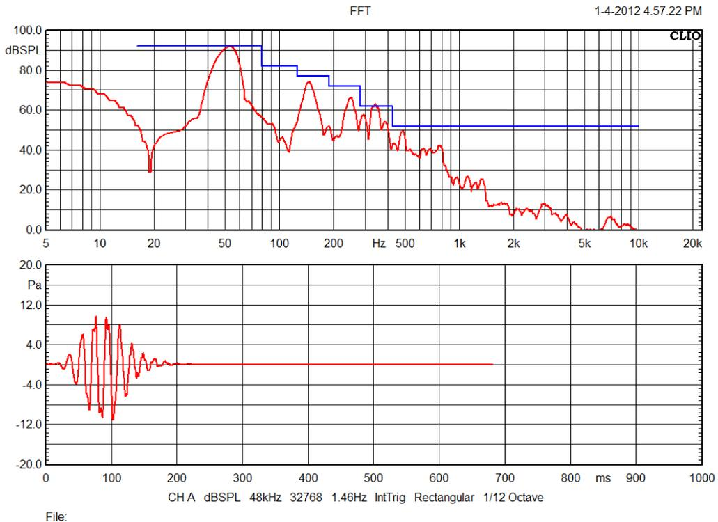
Figure 13: ACE-bass B2-50 - ANSI/CEA-2010 test @ 50 Hz
