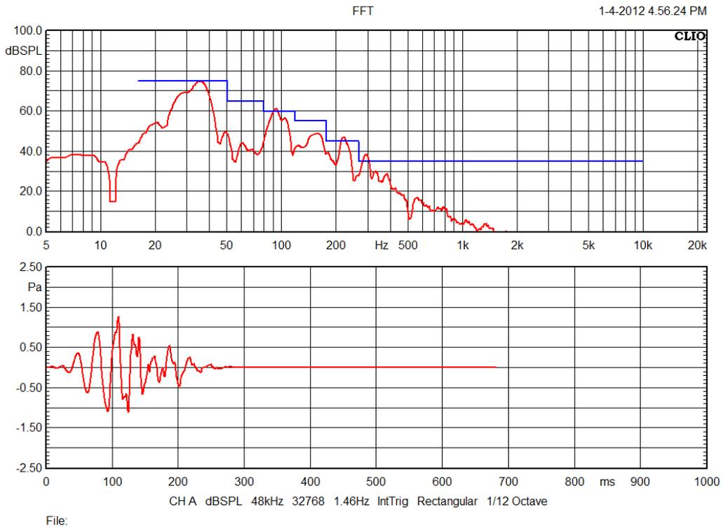
Figure 11: ACE-bass B2-50 - ANSI/CEA-2010 test @ 31.5 Hz
