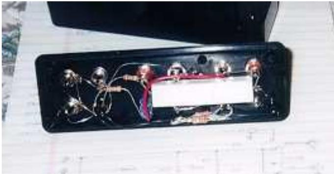
Here is a picture that might help you correctly position the power resistor. There is actually room under it where I mounted some of the calibration reference resistor. Do a trial fit after you mount each resistor so you are sure that everything will go together at the end without bulging the box out.
