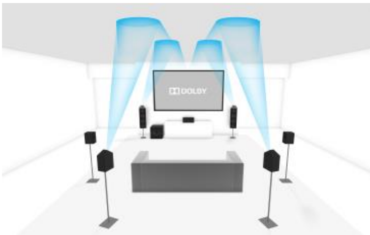
Figure 8: A traditional 7.1 speaker layout with four Dolby Atmos enabled speakers (7.1.4).
