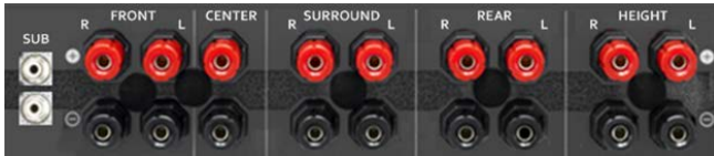
Figure 7: Rear panel of AVR; the height speaker connections are at right.
